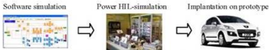
Example of the Power-HIL simulation of a double parallel HEV [4]
